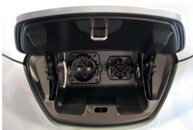
Figure 3. The standard J1772 receptacle (right) can receive charge from Level 1 or Level 2 equipment. The CHAdeMO DC fast charge receptacle (left) uses a different type of connector. Photo by Andrew Hudgins, NREL/PIX 19558
