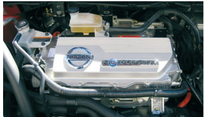
Under the hood of a Nissan Leaf. An EV contains no ICE. Instead, the battery supplies electricity to the electric motor. Photo from Margaret Smith, DOE/PIX 18215
