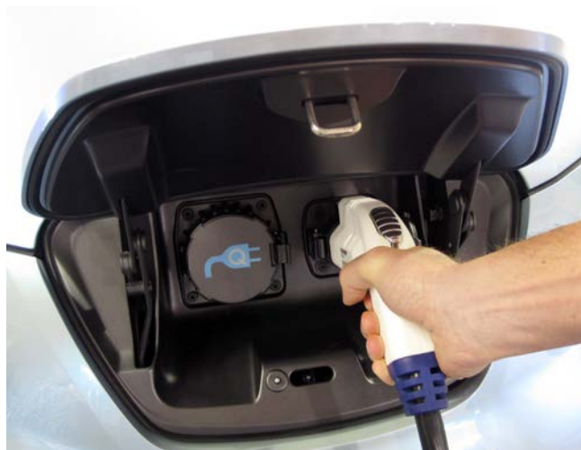
Figure 2. The standard EVSE connector fits into the standard receptacle. Photo by Andrew Hudgins, NREL/PIX 17634
