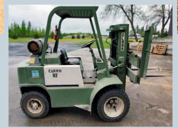
1965 Clark CY70, 7,000 lbs. lifting capacity, propane.
