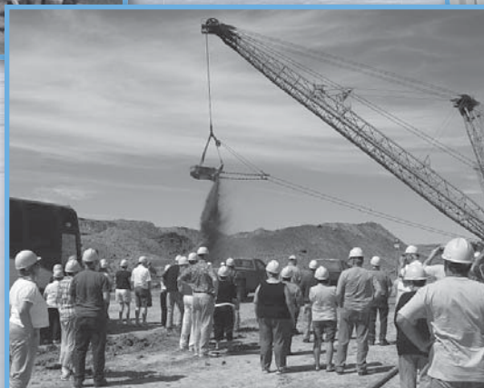
Members watch as the huge dragline gives a demonstration removing overburden from the coal vein at BNI Coal. The Liberty dragline has a 355-foot boom with a 77-cubic-yard bucket.
