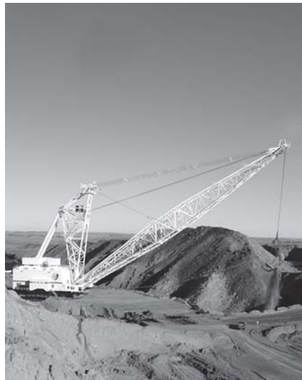
Pictured at left is the new Liberty dragline located at the BNI Coal mine near Center, N.D. The mine produces 4.5 million tons of coal annually for the Milton R. Young Station, which is the primary source of generation for North Star.
