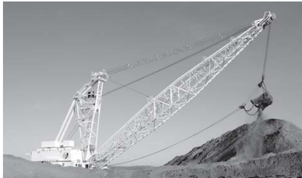
The new Liberty dragline has been in service since October of 2004. Liberty uses 14 direct current motors to perform all of its functions.
